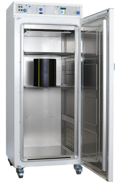
View inside heating oven - pipe sample for heat reversion test inside.
